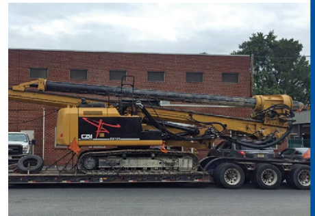
CZM EK125 Drilled Shaft Rig
